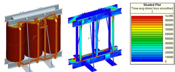
**Fig. 1.** CAD model of a dry-type transformer (left), and the stray loss distribution on its structural components(right).
