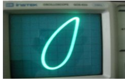
Fig.6. Phase portrait of system R=100 ohm- Limit cycle
